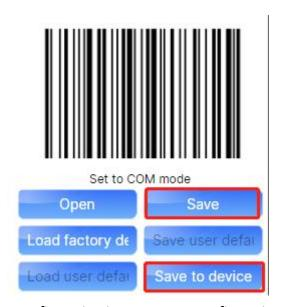
Click "Save" to save all current configuration items as XML configuration files locally. Click "Save to device" to send the modified settings to the device connected to the PC.
